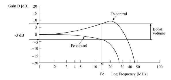
Figure 4.5 Frequency characteristic of programmable filter
